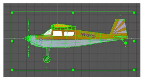
Here you can see the two axes from the front view are on the thrust line and on the wing centre of gravity.
